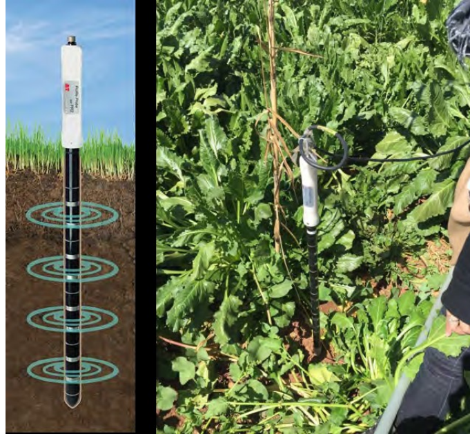
Installation des sondes capacitive
